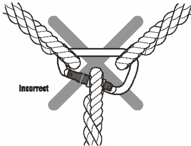
Above: Side and gate loading of a karabiner.
